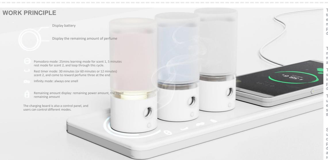
The final product uses methods such as time management, environment establishment, and self-control management to reduce procrastination. The product includes three parts: scent bottle, diffuser and wireless charging board.
