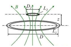
transmitter coil placed at the bottom (L1), receiving coil is located in the top (L2), the coil is embedded into the different electrical devices. L1 is the wireless charging base of nokia, L2 can be understood as the phone itself. Transmitter coil of alternating current (ac) to generate magnetic field, magnetic field by the voltage of receiving coil. The voltage of equipment is used for charging.
