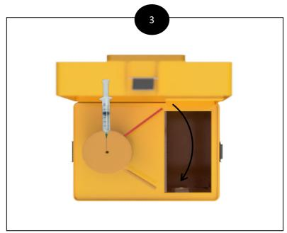
Fingertips or base of the fingers (Make a fist) are used to push the levers together and cut the plastic hub above the needle
