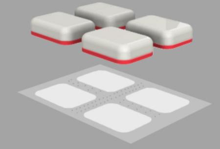
Foam pieces are glued onto base layer fabric and secured by an outer mesh fabric.
