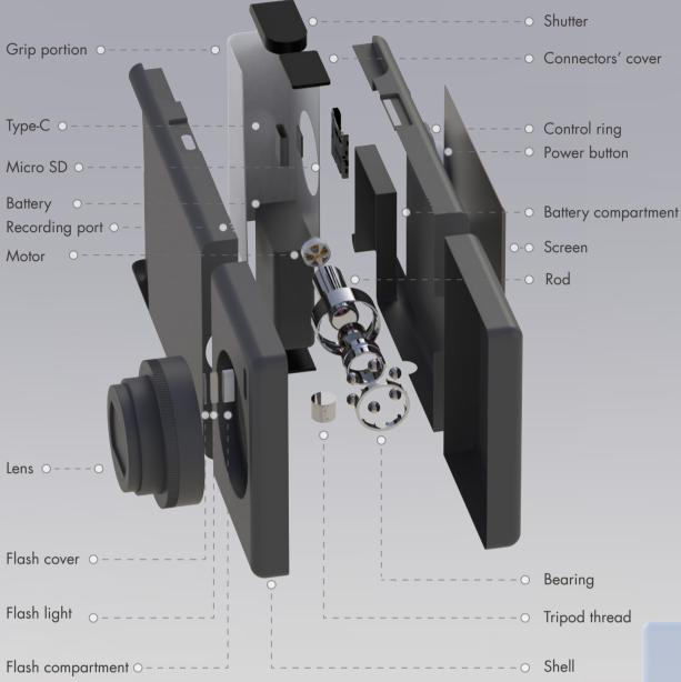
This explosion diagram mainly shows the components of the camera shell and the more characteristic parts, such as the structure of the rotating connecting rod and the built-in small motor used to drive the connecting rod to rotate.
